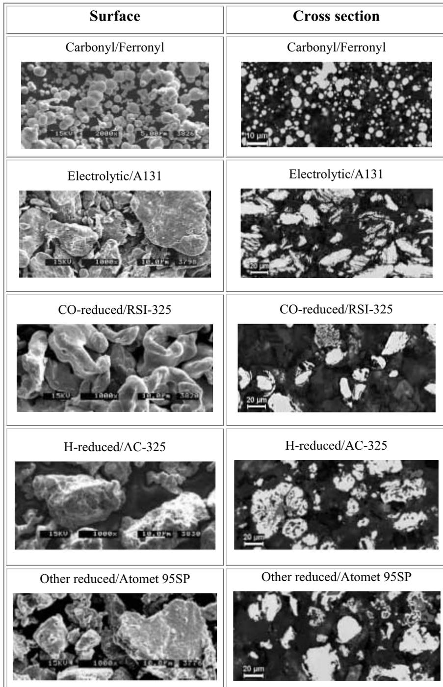
Figure 2: Surface and cross-sectional morphology of elemental iron powders.
